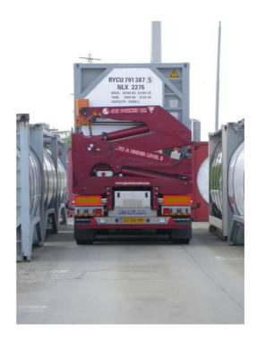
Aisle width can be reduced, that means more containers can be stored on the same block of land.
