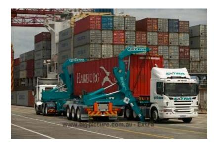
Using the STEELBRO sidelifter together with several skeletal trailers, you can deliver several containers and unload each trailer onto the ground in just 3 minutes. The sidelifter can then re-load the trailer with an empty container from in the area, or the trailer can proceed to the next job.
