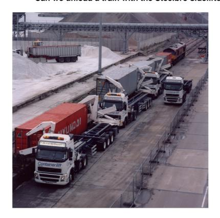
In a small train terminal or in a factory yard, the sidelifter can load or unload trains carrying different kinds of containers.
