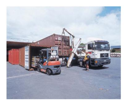
The sidelifter can place the container on the ground, with no need to wait for unloading - and the importer/exporter can unload when he has time.
