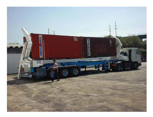
The accessories to connect 2 x 20' containers are supplied with the STEELBRO sidelifter.
