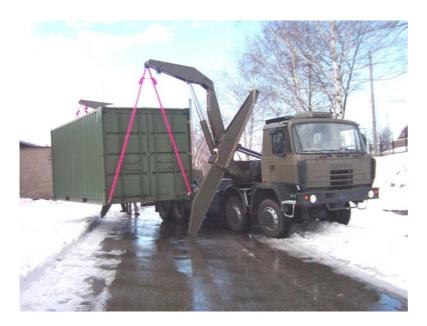
Steelbro chassis cranes mounted on an 8x4 truck are also used by the army especially to carry containers for mobile hospitals; a civilian version on a truck 8 x 4 is also available.
