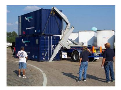
Fully loaded containers can be double-stacked, normal or high cube containers.
