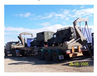
The army uses Steelbro sidelifters intensively to carry vehicles on "flat", tank and normal containers.
