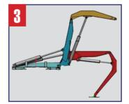
Stabiliser options include Tilt and Extend and Bridge Leg. The SB363 Bridge Leg has angle in feature which is ideal when placing containers close to the wall.
