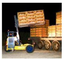
The M10 is the specialist machine for one-side offloading, fitted with forks and extendable boom.
