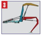
Stabiliser options include **Tilt** and **Extend** and **Bridge Leg**. The **SB363 Bridge Leg** has angle in feature which is ideal when placing containers close to the wall.
