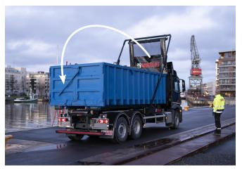
The tarp can be fastened to the mast or in the back of the truck depending on your needs
